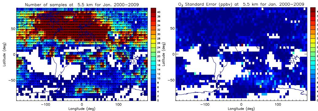
**Fig. 3.** Number of data values and the standard error of the mean for each pixel average in a decadal average map, for January in the mid-troposphere. The standard errors are generally of the order of a few ppbv (right figure), although where data density is low (left figure) they can be higher.
