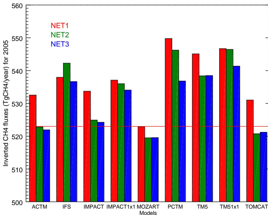
**Fig. 14.** Global methane estimates for every inversion using TransCom model outputs as synthetic observations in three network configurations. Results for NET1, NET2 and NET3 are respectively represented in red, green and blue. The red line exposes the target value of the methane flux at the global scale ( $523 \text{ Tg CH}_4 \text{ yr}^{-1}$ ).
