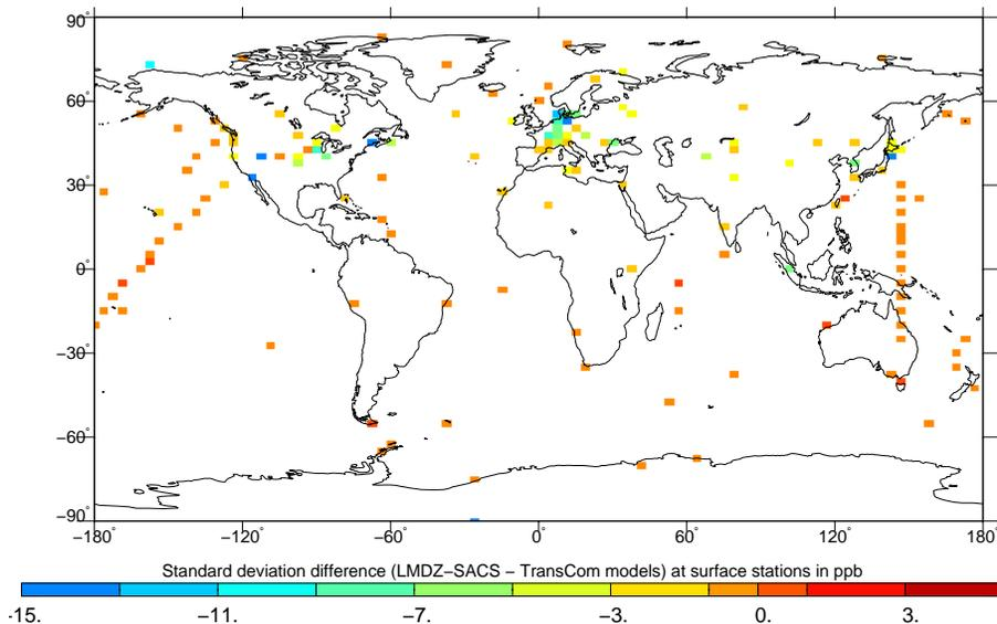
**Fig. 4.** Map of the difference of the “synoptic” standard deviation (STD) computed for  $\text{CH}_4$  mixing ratio simulated by LMDZ-SACS and TransCom models at surface stations ( $\sigma_{\text{LMDZ-SACS}} - \overline{\sigma_{\text{TransCom}}}$ ;  $\overline{\sigma_{\text{TransCom}}}$  is the average of all TransCom models STD). The synoptic STD difference is expressed in ppb.
