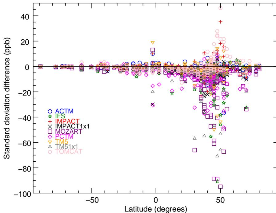
**Fig. 5.** Latitudinal distribution of the “synoptic” standard deviation (STD) difference between LMDZ-SACS and other TransCom models at all surface stations ( $\sigma_{\text{LMDZ-SACS}} - \sigma_{\text{(TransCom model)}}$ ). Each TransCom model is represented by a specific symbol. The STD difference is expressed in ppb.
