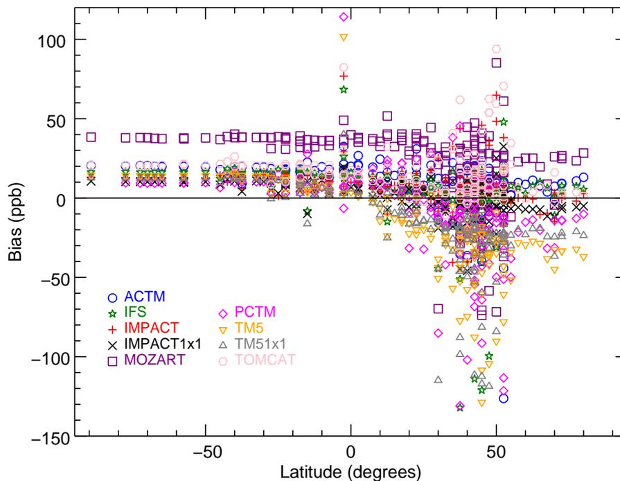
**Fig. 7.** Latitudinal distribution of the bias between  $\text{CH}_4$  mixing ratio simulated by LMDZ-SACS and TransCom models ( $y_{\text{LMDZ}} - y_{\text{TransCom model}}$ ), at all surface stations. Each TransCom model is represented by a specific symbol. The bias is expressed in ppb.
