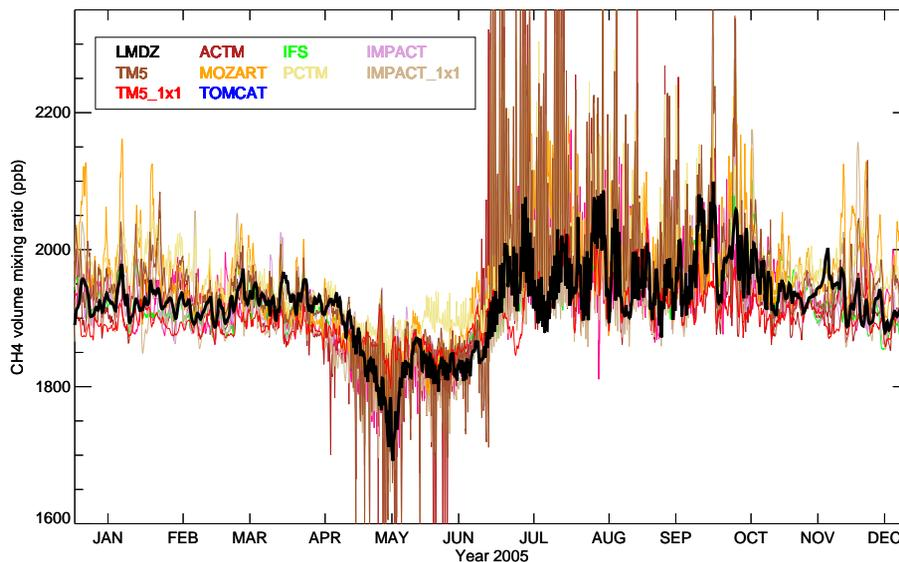
**Fig. 3.** Time series of daily CH<sub>4</sub> mixing ratio at Karasevov (58.25° N, 82.40° E) for 2005. Each TransCom model is represented by a specific color, while LMDZ-SACS is represented by the black line.
