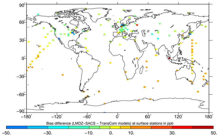
**Fig. 6.** Bias between  $\text{CH}_4$  mixing ratio simulated by LMDZ-SACS and TransCom models ( $y_{\text{LMDZ}} - y_{\text{TransCom}}$ ;  $y_{\text{TransCom}}$  is the average of  $\text{CH}_4$  mixing ratios simulated by all TransCom models) at surface stations. The bias is expressed in ppb.
