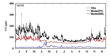
**Fig. 1.** Fig. 1. Time series of observed CO (dots), simulated CO by using anthropogenic emission of EDGAR ver. 4.1 (red), and simulated CO by using biomass burning emission of GFED ver. 3.1 (blue) in 2008.
