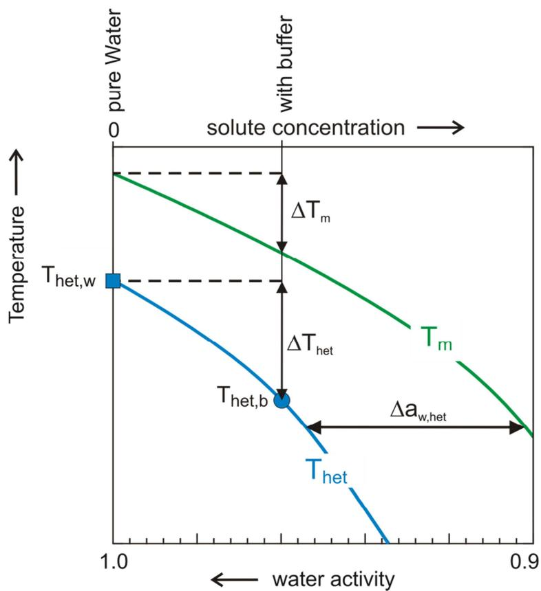
Fig. D: Schematic picture for describing the colligative effect of solutes upon the ice melting point and the heterogeneous ice nucleation temperature (for details see text).
