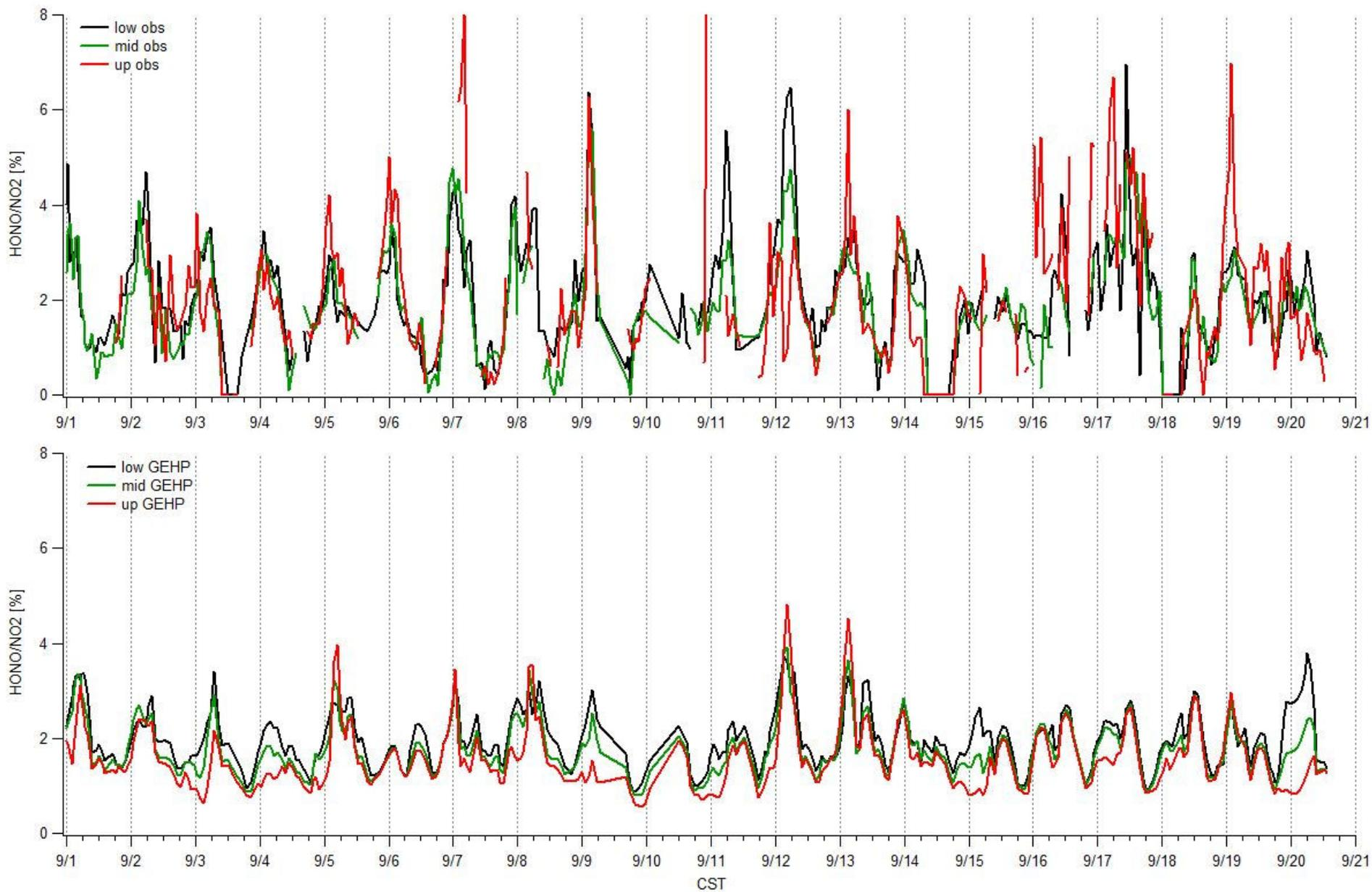
HONO/NO<sub>2</sub> ratio based on measured values (top graph) and simulated values (bottom graph). Different time series correspond to different levels of DOAS measurements.
