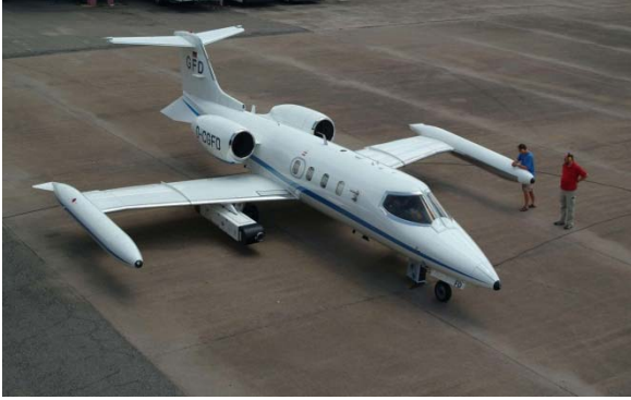
Figure 2: HORUS detection axes are mounted in the wing pod below the wing (© group graphic pool).
