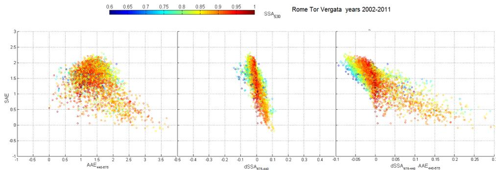
**Fig. 3.** Figure AC3: “Same as Fig.1 but using ten years of AERONET data in Rome (2002-2011). Note that we applied to AERONET level 1.5 all the level 2 criteria except for the AOD threshold
