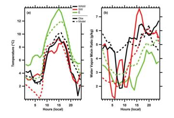
**Fig. 3.** Measured (solid line) and simulated (dashed) daily trends in **(a)** temperature and **(b)** water vapor mixing ratios for the three cases related to air mass origin, i.e. east (E, green), southwest (SW, red) and west northwest (WNW, black).
