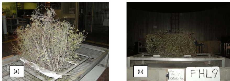
Fig. 1. Fuel bed arrangements (a) : vertical arrangement of Chamise/scrub oak (b) : horizontal arrangements of biomass fuel.
