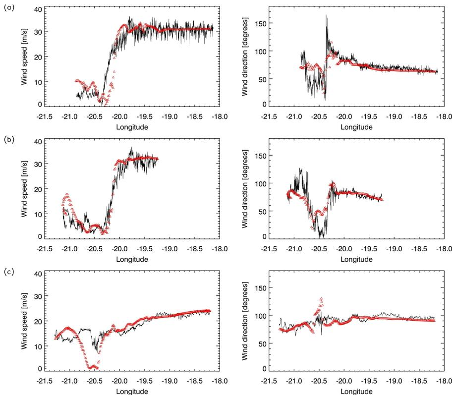
**Fig. 9.** Aircraft measurements (black lines) and G3 simulations from the run MPR (red triangles) at **(a)** 400 m height, **(b)** 700 m height and **(c)** 1900 m height. Wind speed [ $\text{m s}^{-1}$ ] is shown by panels on the left and wind direction [degrees] by panels on the right.
