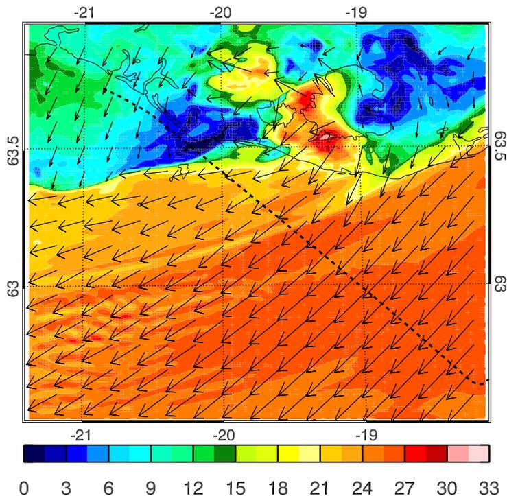
**Fig. 7.** Simulated wind speed [ $\text{m s}^{-1}$ ] (colored shadings) and wind direction (black arrows) at the lowest model level for G3 on 22 February, 12:00 UTC. The dotted line corresponds to leg 5 (400 m height) of the aircraft track. The thin black contours represent land contours.
