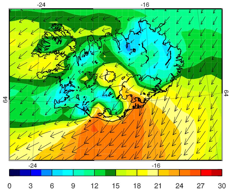
**Fig. 1.** Wind speed [ $\text{m s}^{-1}$ ] (colored shadings) and wind direction (black arrows) from the WRF/Chem simulation at the lowest model level for G1 on 22 February, 12:00 UTC (see Sect. 3.1 for a description of the model configuration).
