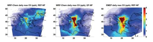
**Fig. 11.** Change in daily maximum near-surface ozone (ppbv) due to forest fire emissions (REF-NF and GF-NF) calculated by WRF-Chem using FINN emissions (left), WRF-Chem using GFED emissions (middle), and EMEP MSC-W using GFED emissions (right) averaged over the summer (JJA) 2007.
