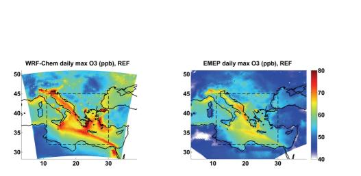
**Fig. 10.** Daily maximum near-surface ozone (ppbv) calculated by WRF-Chem (left) and EMEP MSC-W (right) averaged over the summer (JJA) 2007. The dashed rectangle marks the common EM region.
