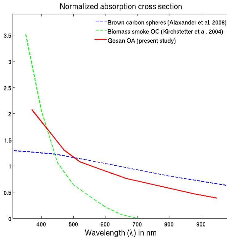
**Fig. 9.** Absorption cross section divided by its average w.r.t. wavelength. Biomass smoke OC refers to organic material in biomass burning aerosols.
