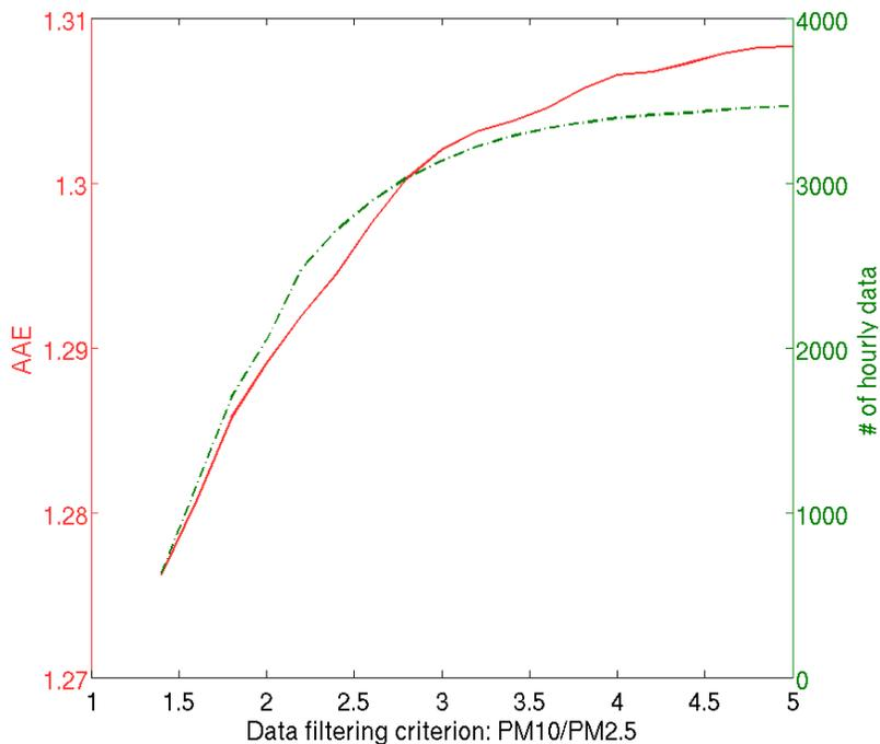
**Fig. 5.** AAE (Absorption Ångström Exponent), as obtained from averaged aethalometer absorption coefficients at 370, 470, 520, 590, 660, 880 and 950 nm. Absorption data are averaged after removing the values corresponding to  $PM_{10}/PM_{2.5}$  being greater than a threshold (i.e. data filtering criterion).  $PM_{10}/PM_{2.5}$  refers to the mass density ratio of  $PM_{10}$  to  $PM_{2.5}$ , and is used as an indicator of dust influence.
