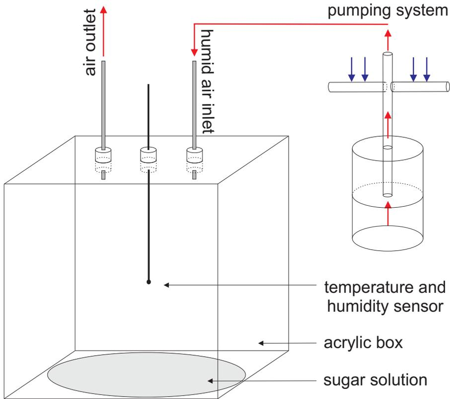
**Fig. 1.** General scheme of the cloud chamber.
