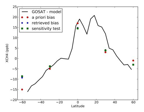
**Fig. 10.** Prior and posterior value of the bias at the five nodes defined in the inversion (60° S, 30° S, 0°, 30° N, and 60° N). Also shown is the difference between the GOSAT GC proxy retrievals and the prior model averaged over the GOSAT data period (June 2009–December 2010).
