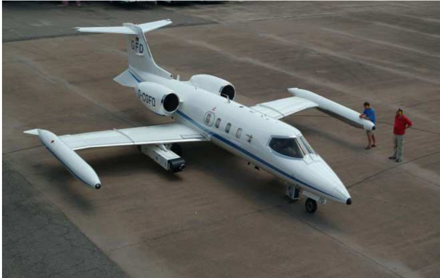
Fig. 2. HORUS detection axes are mounted in the wing pod below the wing (© group graphic pool).
