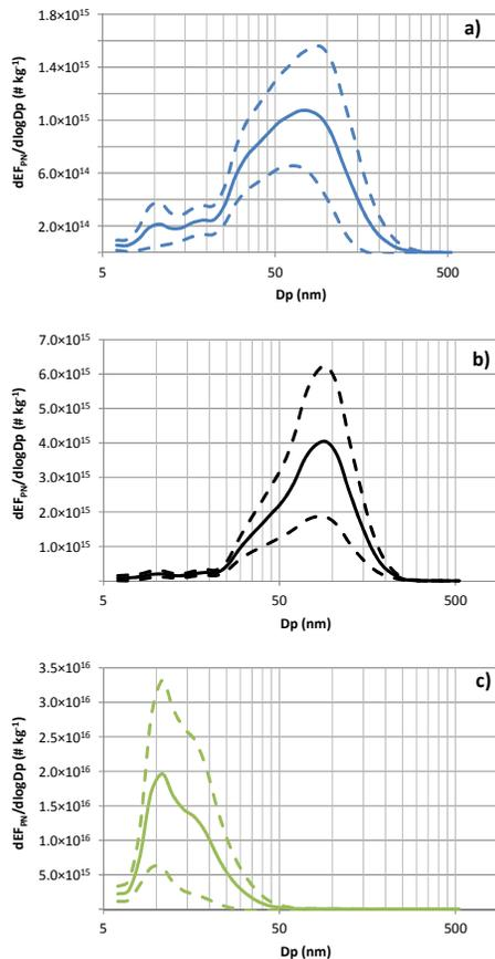
**Fig. 4.** Size-resolved average  $EF_{PN}$  for diesel buses (Euro III–Euro V) with DPF **(a)** without DPF **(b)** and for CNG buses **(c)** for the driving mode *acceleration*. Solid lines averages and dashed lines the statistical 95% confidence interval. For the data presented in graph **(b)** one bus (nr. 34) was excluded, showing much higher size-resolved  $EF_{PN}$  and with a peak size of  $\sim 17 \text{ nm}$ .
