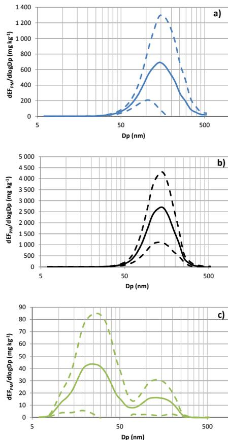
**Fig. 5.** Size-resolved average  $EF_{PM}$  for diesel buses (Euro III–Euro V) with DPF **(a)** without DPF **(b)** and for CNG buses **(c)** for the driving mode *acceleration*. Solid lines averages and dashed lines the statistical 95% confidence interval. For the data presented in graph **(b)** one bus (nr. 34) was excluded, showing a bimodal  $EF_{PM}$  and with peak sizes of  $\sim 30$  nm and  $\sim 190$  nm.
