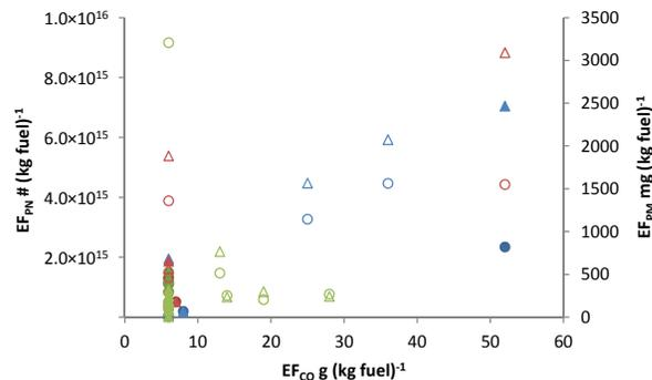
**Fig. 8.**  $EF_{PN}$  (circles) and  $EF_{PM}$  (triangles) versus the EF for  $NO_x$  **(a)** and versus the EF for CO **(b)**. Euro III (blue symbols), Euro IV (red symbols) and Euro V (green symbols). Filled symbols represent buses with DPF installed and unfilled symbols no DPF.
