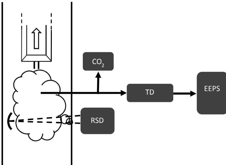
**Fig. 1.** Schematic of the experimental set-up used. EEPS (Engine Exhaust Particle Sizer Spectrometer, Model 3090, TSI Inc.), RSD (Remote sensing device, AccuScan RSD 3000, Environmental System Products Inc.) and TD (Thermodenuder, Dekati).
