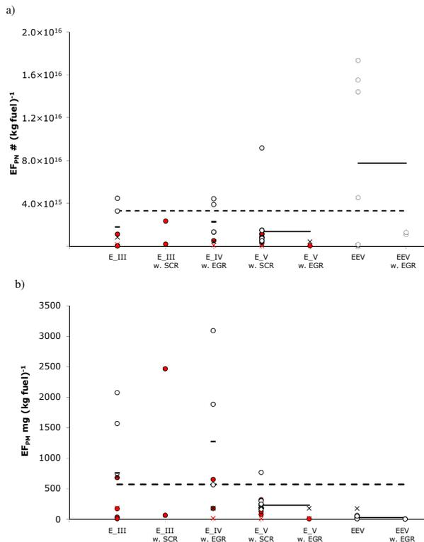
**Fig. 3.**  $EF_{PM}$  (a) and  $EF_{PM}$  (b) for all the buses studied divided into Euro class for the driving mode *acceleration*. Without DPF (white circles), with DPF (red circles), average of all represented Euro classes (dashed line), average of an individual represented Euro class (solid line). Crosses are EFs obtained by the HBEFA 3.1 model with DPF (red) and without (black).
