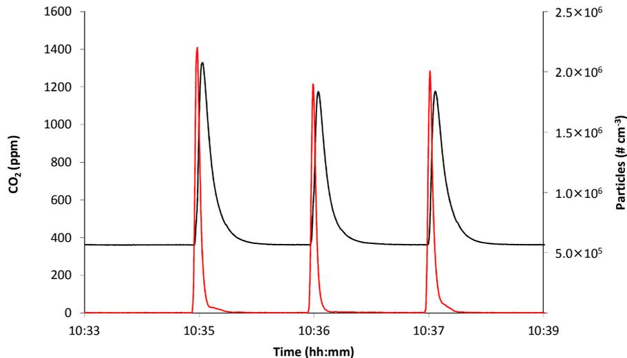
**Fig. 2.** Example of emission signals from three successive individual passages of the same bus in *accelerating mode*. Particle number (red line) and CO<sub>2</sub> concentration (black line).
