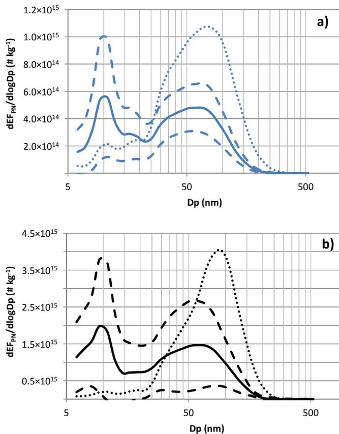
**Fig. 6.** Size-resolved average  $EF_{PN}$  for diesel buses (Euro III–Euro V) with DPF **(a)** without DPF **(b)** for the driving mode *constant speed mode*. Solid lines averages and dashed lines the statistical 95 % confidence interval. Dotted line averages for the *accelerating mode*.
