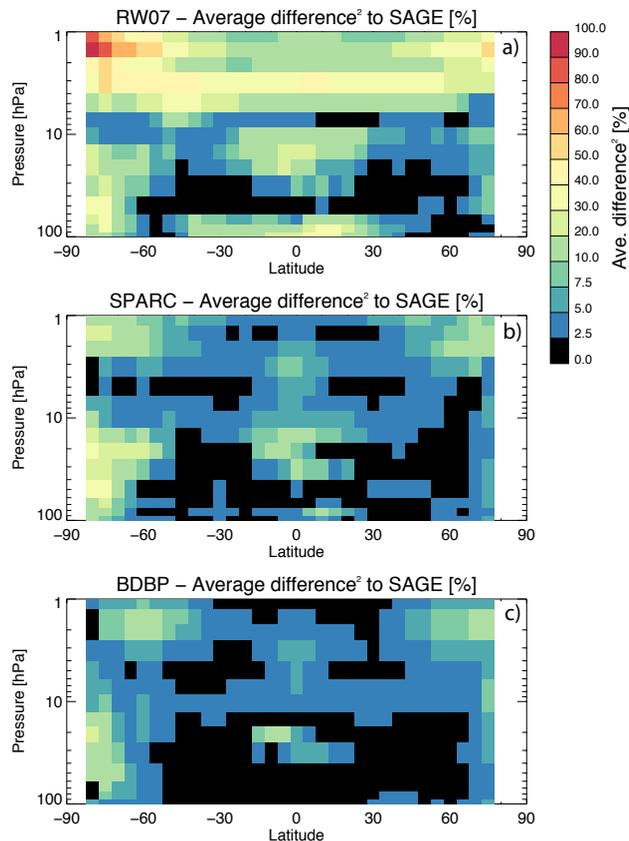
**Fig. 9.** Average squared difference between all available monthly mean SAGE II values for given latitude bands and pressure levels, and **(a)** the RW07 data set, **(b)** the SPARC data set, and **(c)** the BDBP data set, given in percent. Note, that for RW07 at 100 hPa some monthly means are not available between 20° S and 25° N due to missing tropospheric data. Colours changing from black to red indicate a change in average squared differences from 0 % to 100 %.
