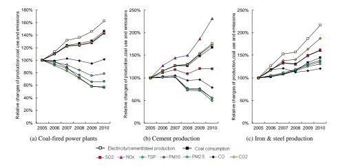
Fig. 6. Relative changes of production, coal consumption and emissions for coal-fired power plants (a), cement plants (b) and iron and steel plants (c) from 2005 to 2010. Note the scales are different for the three panels.
