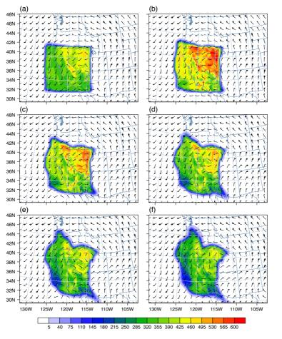
**Fig. 4.** Bin 2 sulfate aerosol mixing ratios  $[\mu g kg^{-1} \text{ of dry air}]$  and wind barbs (kts) at the level of the injection on 23 July at hours (a) 08:00 LT, (b) 10:00 LT, (c) 12:00 LT, (d) 14:00 LT, (e) 16:00 LT, and (f) 18:00 LT.
