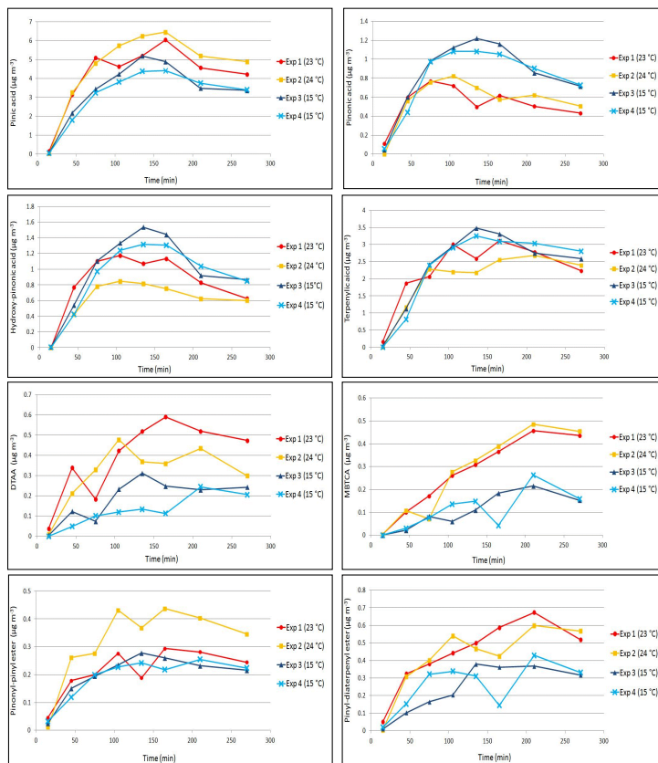
Fig. 1. Concentration profiles during smog-chamber experiments. ● Experiment 1 (23°C), ■ Experiment 2 (24°C), ▲ Experiment 3 (15°C), × Experiment 4 (15°C). No correction for wall losses has been applied.
