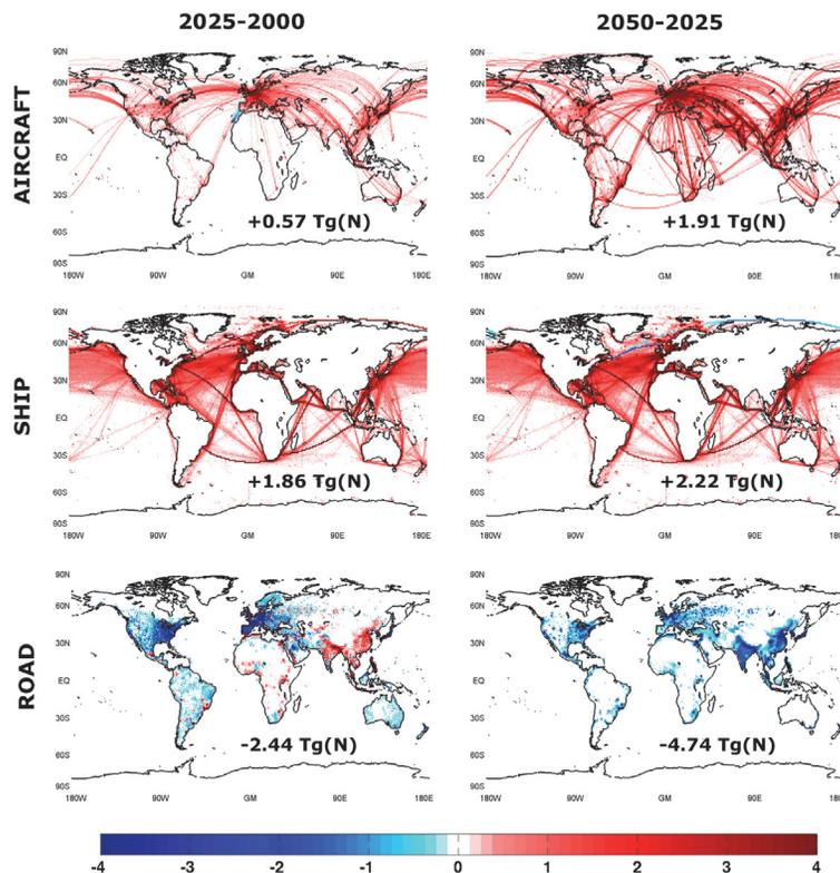
**Fig. 1.** Spatial distribution of the absolute difference in  $\text{NO}_x$  emission flux for the SRES A1B scenario (units:  $10^{13}$  molecules  $\text{NO}_2 \text{ m}^{-2} \text{ s}^{-1}$  for AIRCRAFT and SHIP;  $10^{14}$  molecules  $\text{NO}_2 \text{ m}^{-2} \text{ s}^{-1}$  for ROAD).
