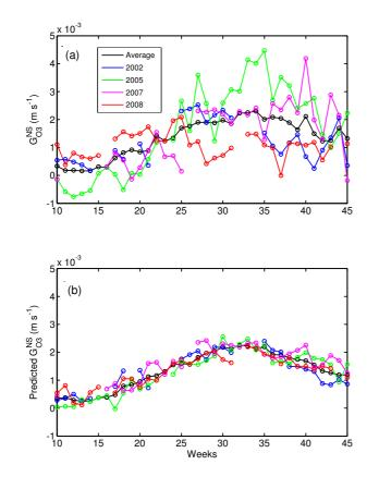
**Fig. 9.** Weekly average non-stomatal  $O_3$  conductance for day-time conditions (solar elevation angle > 10°) as observed **(a)** and predicted by using the partial least squares technique **(b)**.
