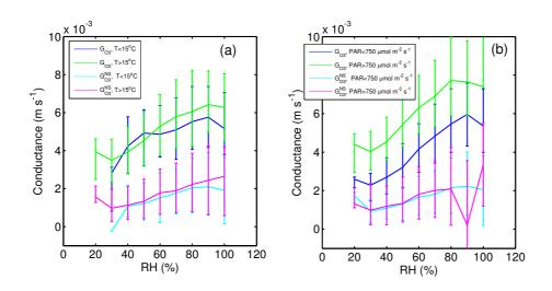
**Fig. 5.** Day-time (elevation angle of sun > 10°) ozone conductance as a function of RH during weeks 25–34. 15 °C and 750  $\mu$ mol m<sup>-2</sup> s<sup>-1</sup> were used as the values to separate high and low temperature (a) and PAR (b) conditions. Medians of 30 min averages observations together with quartiles are presented.
