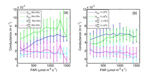
**Fig. 6.** Day-time (elevation angle of sun > 10°) ozone conductance as a function of PAR during the peak of the growing season weeks 25-34. 70% and  $15^{\circ}$ C were used as the values to separate high and low relative humidity (**a**) and temperature (**b**) conditions. Medians of 30 min averages observations together with quartiles are presented.
