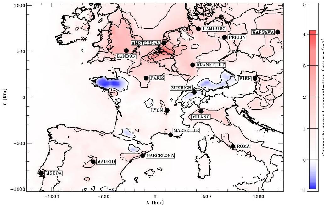
**Fig. 1.** Difference in monthly average aerosol concentration ( $\mu\text{g m}^{-3}$ ) between two simulations with a 15% emission reduction of either NOx or NH<sub>3</sub> in January 2006 for the European domain.
