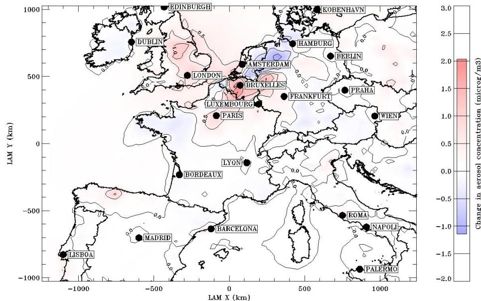
**Fig. 2.** Difference in monthly average aerosol concentration ( $\mu\text{g m}^{-3}$ ) between two simulations with a 15% emission reduction of either NOx or NH3 in June 2006 for the European domain
