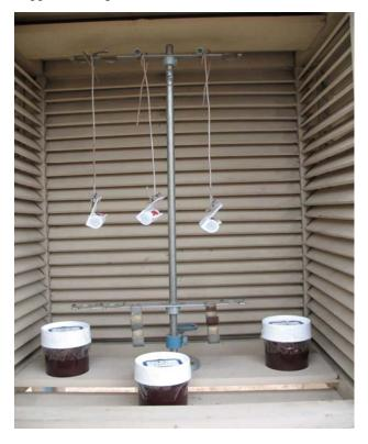
The exposed samplers and field samplers of  $NH_3$ ,  $SO_2$  and  $NO_2$  in the thermometer screen at the site.
