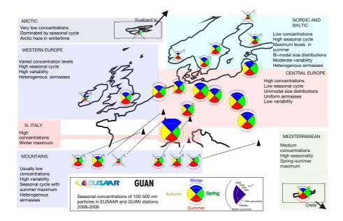
Fig. 15. Overview of EUSAAR and GUAN station measurements – spatial distribution of particle number concentrations on particle (in cm<sup>-3</sup> STP). The coloured areas are relative to the median concentration observed in each season, and the lower and higher arcs show 16th and 84th percentile concentrations. The colours and location of the segments show different seasons. The locations of the stations are approximate. Stations ZEP (Arctic) and FKL (Mediterranean) are located in inserts.
