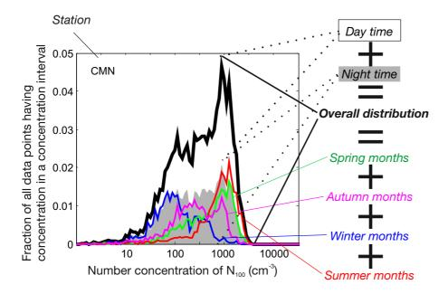
**Fig. 8.** Example of the number concentration histograms used in Figs. 9–11. The black line shows the histogram (with log-evenly distributed bins) of all available data from the station. The seasonal histograms are normalized to total amount of available data; they sum up to the total histogram value. The shaded area shows the similarly normalized histogram of only night-time samples. The white area above is the fraction of the total histogram which was from the day-time samples.
