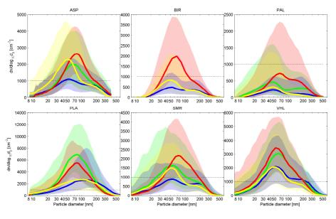
**Fig. 4.** Median distributions (solid line) and 16th and 84th percentile distributions (shaded areas) divided by seasons at Nordic and Baltic (PLA) stations. The black dotted line shows the 1000 particles cm<sup>-3</sup> size distribution value to help the eye on the concentration levels. Blue line and shading denote winter, green line and shading spring, red line and shading summer and yellow line and shading autumn months datasets.
