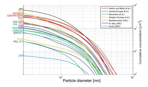
Fig. 14. Cumulative number concentration of the median size distributions at EUSAAR and GUAN stations. The summation was done starting from the largest available size. The plot shows how much particles were above each diameter in the median size distribution.
