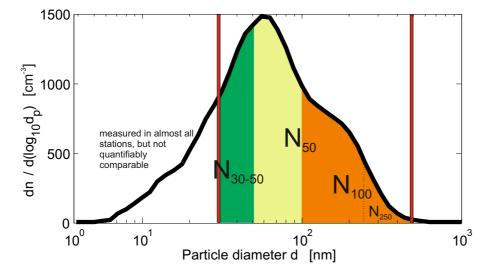
**Fig. 1.** Size regions used in the analysis. The red lines show the size cut-offs from 30 nm to 500 nm. The green area shows the region used to calculate  $N_{30-50}$ , the orange area  $N_{100}$  and the total area of orange and olive are the  $N_{50}$  ( $N_{100}$  is part of  $N_{50}$ ).  $N_{250}$  concentration (Appendix B) is shown in dotted line.
