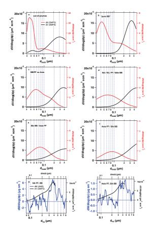
Fig. 13. (a-f) Lognormal fits for SMPS number and volume size distributions for all five plume categories and all non-plume periods. (g,h) AMS mass and SMPS volume size distributions (lognormal fits) for an Asian FF and Siberian BB influenced plume (Plume IV), and a North American FF and BB influenced plume. The AMS data has been smoothed with a sliding average over 10 size bins.
