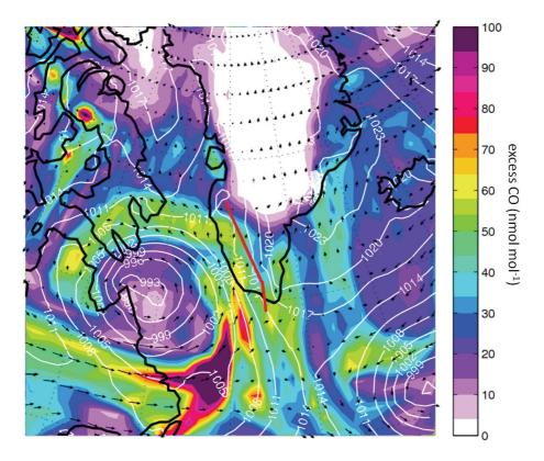
Fig. 2. Low pressure system west of Greenland on 8 July at 15:00 UTC at 5000 m altitude. The colour-code denotes FLEXPART derived excess CO mixing ratio in nmol mol<sup>-1</sup>, the white contours represent surface pressure levels from 980 to 1030 hPa in 3 hPa intervals.
