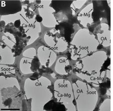
**Fig. 7.** TEM image of smoke samples from **(a)** garbage burning and **(b)** mixture of garbage burning and crop residue burning. The black horizontal bar at the base of each image indicates 1 micron. See Sect. 3.2 for discussion.
