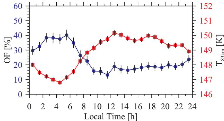
**Fig. 8.** Diurnal variation of NLC occurrence determined from ALOMAR RMR-lidar ( $\beta_{\max} > 4$ , blue circles) and temperature at 83 km altitude during times of lidar measurements as calculated by LIMA (red squares) for the integrated data set from 1997 to 2010. Vertical bars indicate confidence limits for the occurrence at 95%-level and errors of the mean temperatures.
