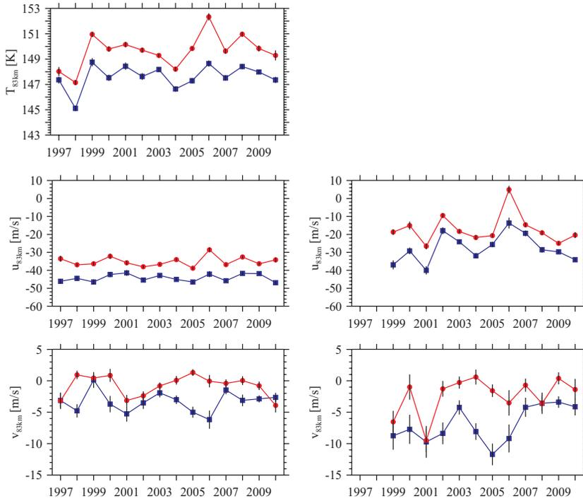
**Fig. 7.** Seasonal mean temperature (top), zonal (middle) and meridional (bottom) wind at 83 km altitude above ALOMAR as calculated by the LIMA-model (left) and measured by the ALOMAR MF-radar (right). Data are based on hourly mean values. Only hours with ALOMAR RMR-lidar measurements are taken into account (long-term data set). Data are separated for confirmed absence (red circles) and presence ( $\beta_{\max} > 4$ , blue squares) of NLC. Vertical bars are error of the means.
