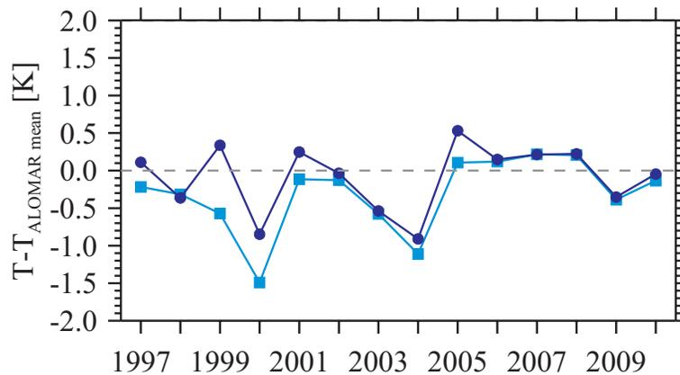
**Fig. 9.** Seasonal mean sampling of temperature at 83 km altitude during ALOMAR RMR-lidar measurements as determined by LIMA. Temperatures calculated solely for hours with lidar measurements are compared to entire means from 1 June to 15 August. Sampling curves are calculated for two data sets: long-term (blue circles) and high-sensitivity (light blue squares).
