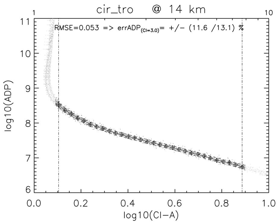
**Fig. 6.** Correlation diagram between  $\log_{10}(CI_A)$  and  $\log_{10}(ADP)$  with ADP in  $\mu\text{m}^2 \text{cm}^{-2}$  for tropical CSDB spectra at 14 km tangent height (dots). Roots mean square error bars with respect to a fitted 4th order polynomial are superimposed.
