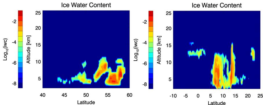
**Fig. 7.** Latitude-altitude cross section of ice water content in  $\text{g m}^{-3}$  and log10 scale from ECMWF data. These data were input to the radiative transfer calculation for Scenario 1 and 2 (left/right: mid and tropical latitudes).
