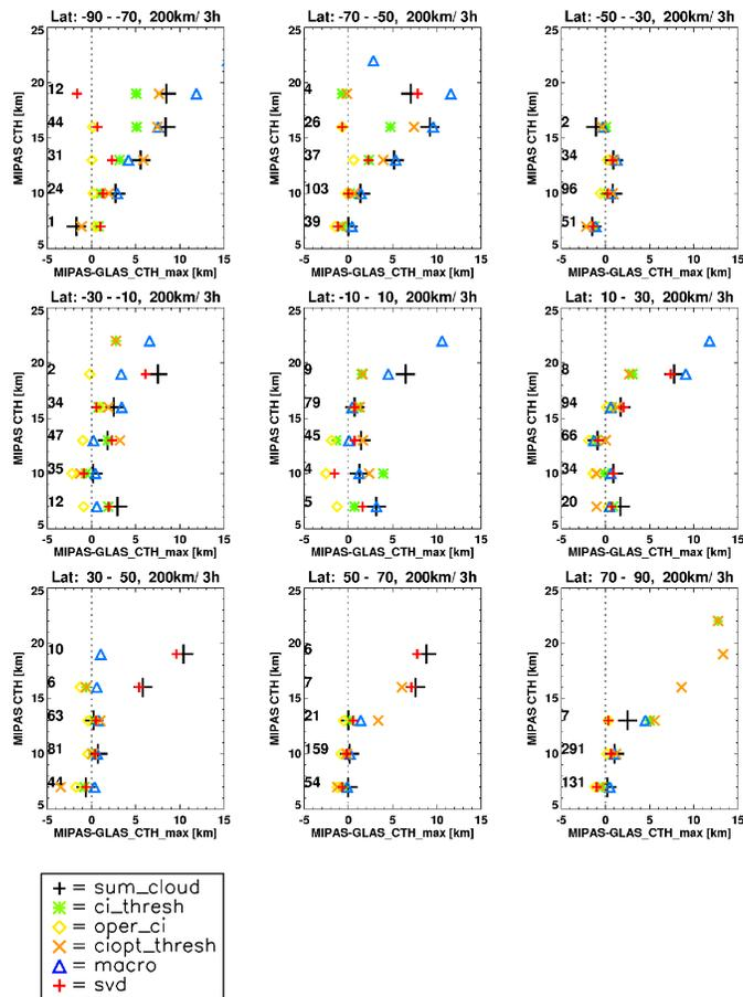
**Fig. 15.** Altitude-binned differences of cloud top heights between the various MIPAS detection methods and the GLAS lidar co-incidences (200 km/3 h). Black number represents the number of both-cloudy events for the parameter SUM\_CLOUD.
