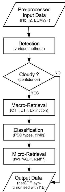
**Fig. 1.** Overview of the MIPclouds processing scheme. The pre-processing of the input data is part of the original cloud processor. (\*) Ice water path (IWP) is an integrated quantity over the limb path, as well as for the area density path (ADP). (\*\*) For the current processor version, retrieval results of  $R_{\text{eff}}$  are not recommended for scientific analyses, further investigations and improvements on the algorithms are necessary.
