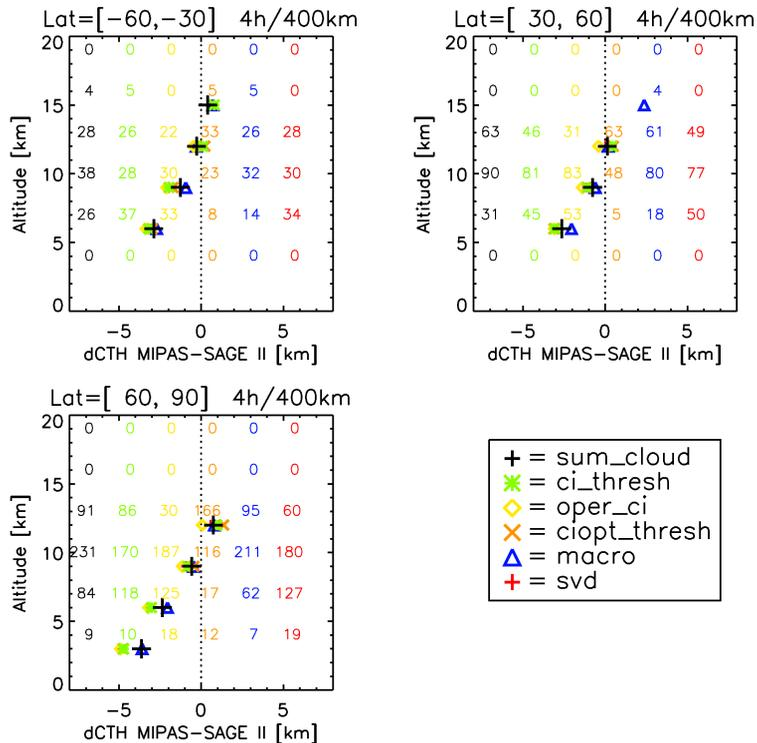
**Fig. 14.** Mean difference in CTH between MIPAS and SAGE II for coincident cloudy profile measurements between October 2002 and March 2004 on a 3 km altitude grid and three latitude bins (60° S–30° S, 30° N–60° N, and 60° N–90° N). Coloured symbols indicate the different MIPAS detection methods and the coloured numbers represent the counts of CTHs for MIPAS for the corresponding altitude bin and detection method.
