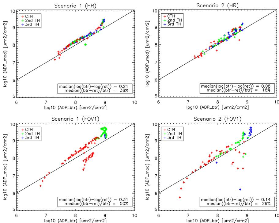
**Fig. 11.** Retrieved ADP versus “real” ADP values at the detected CTH in blind test data fields for Scenario 1 and 2 (left/right). Top figures show the high-resolution (HR) and the bottom figures the FOV convolution results.
