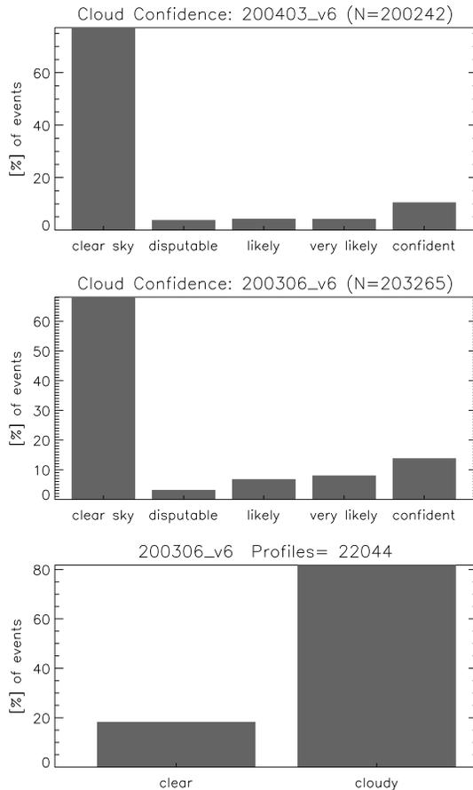
**Fig. 4.** Probability distribution in percentage of the normalised cloud confidence flag for all spectra analysed for March 2004 (top) and June 2003 (middle) in the altitude range 3 to 33 km. Bottom figure shows the corresponding number of cloudy and non-cloudy profiles for the June 2003 distribution shown above.
