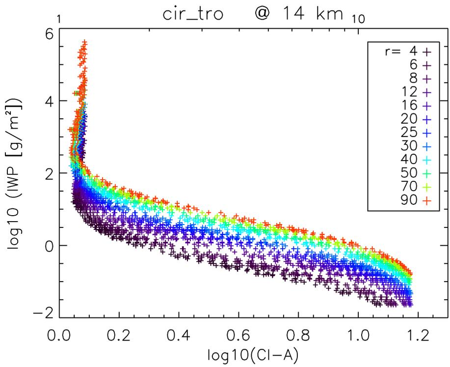
**Fig. 5.** Correlation diagram between  $CI_A$  and the cirrus IWP (both parameters in  $\log_{10}$  space) for tropical CSDB spectra at 14 km altitude. The varying effective radius in units of  $\mu\text{m}$  is colour coded.
