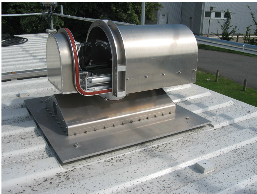
Fig. 1. The mounted hutch cover in its opened position. The red seals can be pressurized to close the hutch hermetically. The solar tracker mirrors and the pneumatic cylinder that controls the movement of the hutch cover are located inside the hutch.
