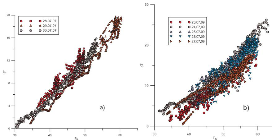
**Fig. 3.** The temperature differences  $\delta T$  between the ground surface temperature  $T_s$  (°C) and temperature at 0.2 m: **(a)** data of 28–30 July 2007, **(b)** data of 23–27 July 2009.
