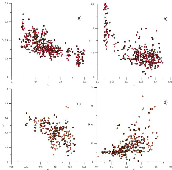
**Fig. 9.** Deviation of the 0.5-m aerosol mass concentration from the background value at 2 m (2007) or 1.5 (2009) ( $\mu\text{g m}^{-3}$ ) for particles 0.15–0.5  $\mu\text{m}$  in size as a function of the friction velocity  $u_*$ : **(a)** – 28 July 2007, **(b)** – 30 July 2007, **(c)** – 27 July 2009, **(d)** – 20 July 2010.
