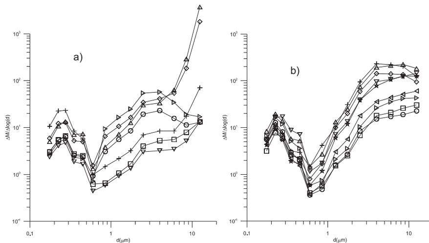
**Fig. 2.** Daytime-averaged at 2 m distributions **(a)** for 2007, **(b)** for 2009 of aerosol particles mass concentrations with the particles size; inserts: the daytime-averaged horizontal velocity at 2 m (for 2007) and 2.2 m (for 2009).
