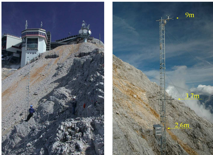
Fig. 3. Photographs showing the two masts, one on the northern side (left panel) and the other one on the southern side (right panel) of the ridge. The view is from the southwest looking upwards towards the summit of Mt. Zugspitze. Measurements at each mast are taken at two altitudes, namely at z = 3.7 m and z = 9 m above ground.
