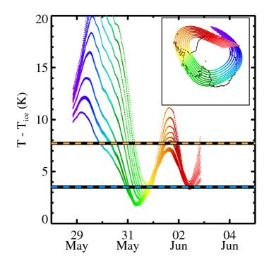
**Fig. 18.** Back trajectories calculated for the 500 K isentropic level for a MIX2 PSC detected along orbit track 12 on 2 June 2008 (see Figs. 12f and 13f) in the polar stratospheric belt showing the passage over the Antarctic Peninsula and the synoptic-scale temperature history. The colors in the inset map indicate the time along the trajectory. The yellow-black and cyanblack dashed lines indicate the NAT existence temperature and STS formation temperatures, respectively.
