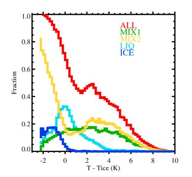
**Fig. 3.** Fraction of positive PSC detections compared to all CALIOP observations as a function of temperature relative to the ice frost point for the PSC types classified in Fig. 2, MIX1 (green line), MIX2 (yellow line) LIQ (cyan line) and ICE (blue line). The sum of the detections of all four PSC types (red line) is also indicated.
