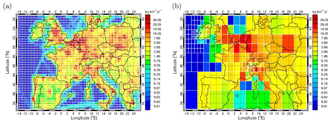
**Fig. 3.** CO emissions according to EMEP/CEIP (<http://www.ceip.at/>) inventory and reduced by a factor 1000 to match the range of halocarbon emissions. **(a)** Emissions on regular  $0.5^\circ \times 0.5^\circ$  grid. **(b)** Emissions on reduced grid with 224 cells used for the inversion.
