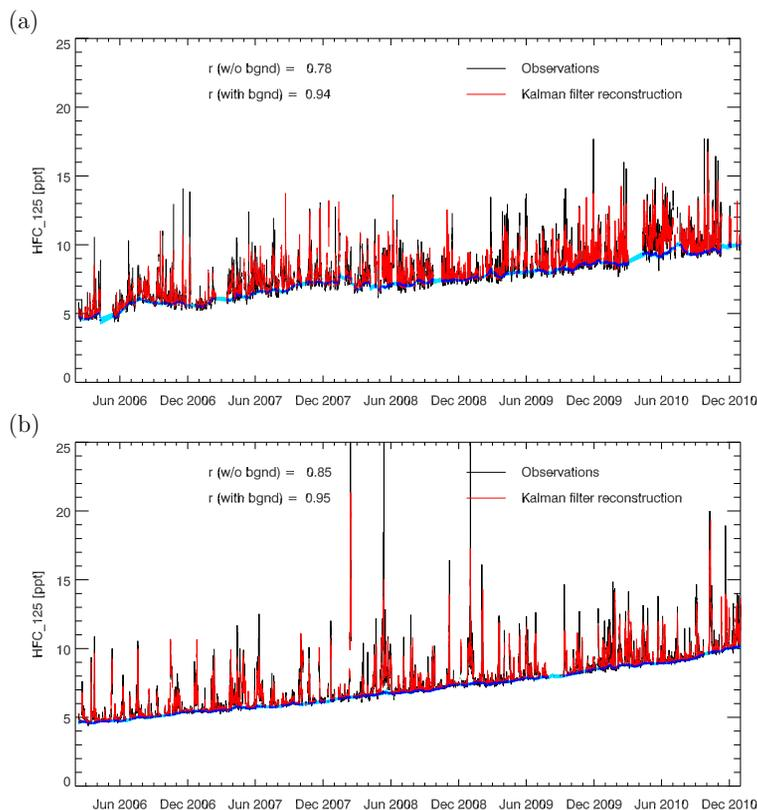
**Fig. 8.** Comparison of observed (black) and simulated (red) time series at **(a)** Jungfrauoch and **(b)** Mace Head from 2006 to 2010. Dark blue lines are smooth backgrounds estimated by the Kalman filter and light blue bands corresponding uncertainty ranges.
