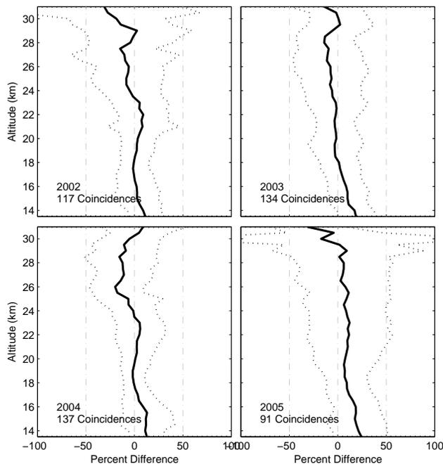
**Fig. 4.** The mean and standard deviation of the percent difference of all OSIRIS and SAGE III coincidences over the four years of mission overlap, 2002–2005. Top left panel shows the results for 117 coincident measurements in 2002; top right panel shows the results for 134 coincident measurements in 2003; bottom left panel shows the results for 137 coincident measurements in 2004; and, bottom right panel shows the results for 91 coincident measurements in 2005.
