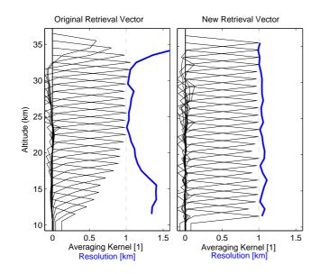
**Fig. 2.** The averaging kernel in black and resolution in terms of Full Width Half Maximum (FWHM) in blue for a simulated aerosol retrieval using lines-of-sight spaced 1 km in tangent altitude. The left panel shows the result when using the retrieval vector defined in Eq. (1). The right panel shows the improvement when using the retrieval vector defined in Eq. (4).
