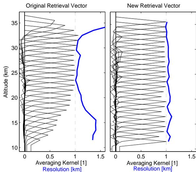
**Fig. 2.** The averaging kernel in black and resolution in terms of Full Width Half Maximum (FWHM) in blue for a simulated aerosol retrieval using lines-of-sight spaced 1 km in tangent altitude. The left panel shows the result when using the retrieval vector defined in Eq. (1). The right panel shows the improvement when using the retrieval vector defined in Eq. (4).
