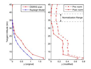
**Fig. 1.** The stratospheric aerosol measurement vector, y. The left panel shows y as calculated according the original algorithm for a typical OSIRIS scan in red as well as y for a model calculation of an aerosol-free atmosphere in blue. The right panel shows the modified version of y, before and after the normalization (with red and dashed red lines according to Eqs. (3) and (4) respectively).
