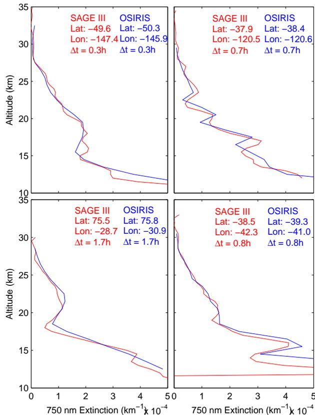
**Fig. 3.** Four coincident SAGE III and OSIRIS aerosol extinction coefficient measurements. SAGE III measurements at 755 nm are shown in red and OSIRIS measurements at 750 nm are shown in blue. The latitude, longitude of each measurement and the time difference between each coincident SAGE III and OSIRIS measurement are given in each corresponding plot.
