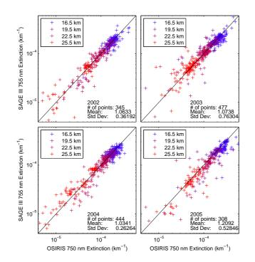
**Fig. 5.** Comparison of OSIRIS and SAGE III aerosol extinction coefficient at four altitude levels: 16.5, 19.5, 22.5 and 25.5 km. Each panel represent one of the four years of overlapping measurements: 2002 in top left, 2003 in top right, 2004 in bottom left and 2005 in bottom right. The mean and standard deviation given in the plots are calculated based on the ratio given in Eq. (6).
