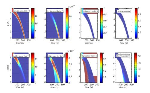
Fig. 10. Model run with  $E_{agg}$  set to zero (top plots) and  $E_{agg}$  set to unity (bottom plots).
