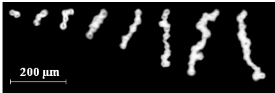
Fig. 10. Typical examples of chain-like aggregates ice crystals from 2 up to 15 individual frozen droplets.
