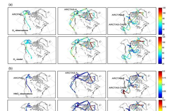
**Fig. 3.** (a)  $O_3$  and (b) HNO $_3$  mixing ratios (ppb) observed during the ARCPAC (3 to 23 April 2008), the ARCTAS-A (1 to 19 April 2008) and the ARCTAS summer (18 June to 13 July 2008) campaigns (ARCTAS-CARB and ARCTAS-B) (a) compared to model values (b) sampled along the flight track at the same time, location and altitude of the observations. The flight tracks extend from 0 to 7 km for ARCPAC, from 0 to 9 km for ARCTAS-CARB and from 0 to 12 km for ARCTAS-A and -B.
