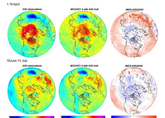
**Fig. 13.** Mean  $O_3$  columns (molecules/cm2) from ground to 300 hPa during the spring (from 1 to 19 April) and summer (from 18 June to 13 July) campaign periods, observed by the IASI satellite instrument and simulated by MOZART-4, smoothed according to the averaging kernels of the IASI observations. The percent differences between the observations and the model results (calculated as [(model-obs.)/obs.]·100 %) are shown on the right panel.
