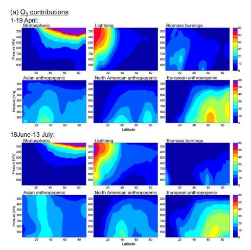
**Fig. 10.** Vertical and latitudinal distributions of the relative contributions (%) to  $O_3$  (a) and HNO3 (b) concentrations during the spring (from 1 to 19 April) and summer (from 18 June to 13 July) ARCTAS campaigns, as simulated by MOZART-4.
