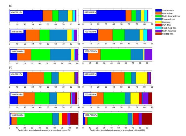
**Fig. 8.** Partitioning of principal sources to  $O_3$  (left) and HNO $_3$  (right) in altitude bands of ground-700 hPa, 700–450 hPa and 450–300 hPa along the ARCTAS spring **(a)** and summer **(b)** flight tracks (from 18 June to 13 July), as simulated by MOZART-4, expressed in percentage (%) of the total.
