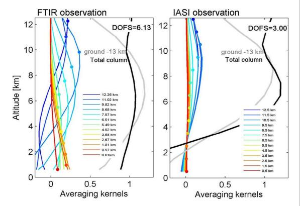
**Fig. 2.** Typical FTIR (left) and IASI (right)  $O_3$  averaging kernels in partial column units (mol cm<sup>-2</sup>/mol cm<sup>-2</sup>) for different retrieved layers for  $O_3$  at Eureka (10 July).
