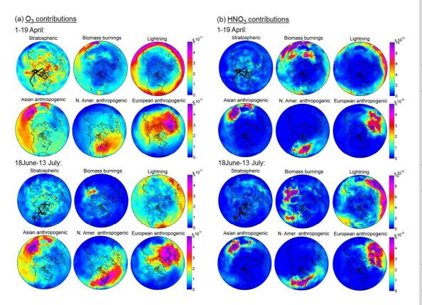
**Fig. 9.** Principal contributions to  $O_3$  (a) and to  $HNO_3$  (b) columns (molecules cm<sup>-2</sup>) from the ground to 300 hPa during spring (from 1 to 19 April) and summer (from 18 June to 13 July) ARCTAS campaigns, as simulated by MOZART-4. The flight tracks corresponding to these periods are superimposed in black on the stratospheric contribution plots.
