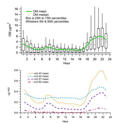
Fig. 2. (a) Box plot of AMS OM ( $\mu$ g m<sup>-3</sup>) by hour, and (b) average concentrations of selected m/z (43, 44, 57, and 60) by hour.
