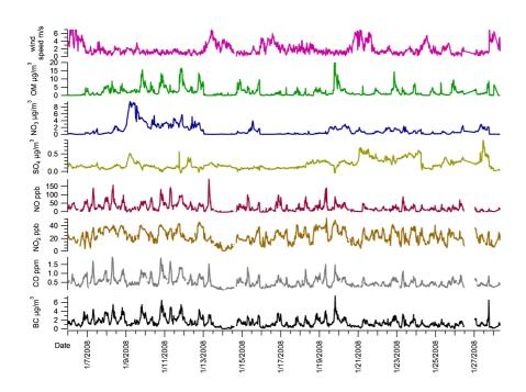
Fig. 3. Time series of wind speed  $(m s^{-1})$ , AMS OM  $(\mu g m^{-3})$ , AMS nitrate, AMS sulfate, Aethalometer  $^{\text{TM}}$  BC ( $\mu\text{g m}^{-3}$ ), CO (ppm), NO (ppb) and NO $_2$  (ppb). Major tick marks indicate midnight for each day.
