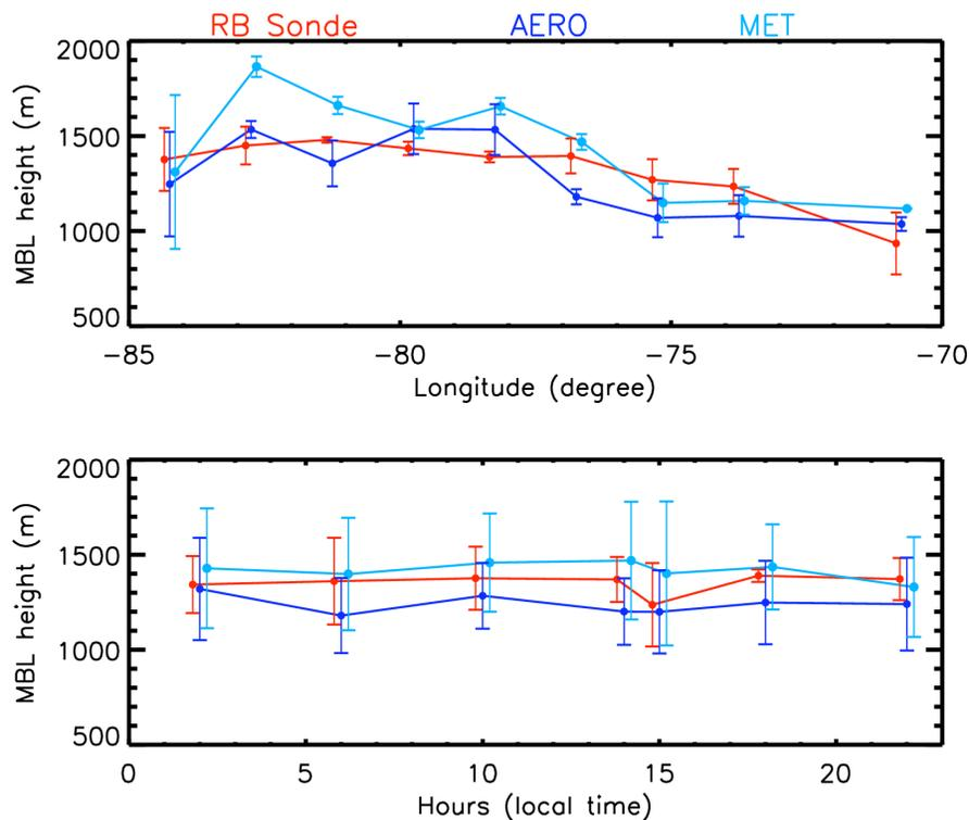
**Fig. 2.** Longitudinal and diurnal variations of the MBL heights derived from RB radiosondes measurements (red), and from the AERO (blue) and MET (light blue) simulations. The MBL heights are determined from temperature profiles in combination with humidity profiles.
