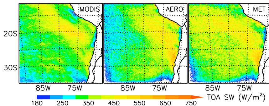
**Fig. 9.** Top of the atmosphere (TOA) outgoing shortwave (SW) radiation fluxes measured by CERES (Terra) and those simulated in the AERO and MET simulations.
