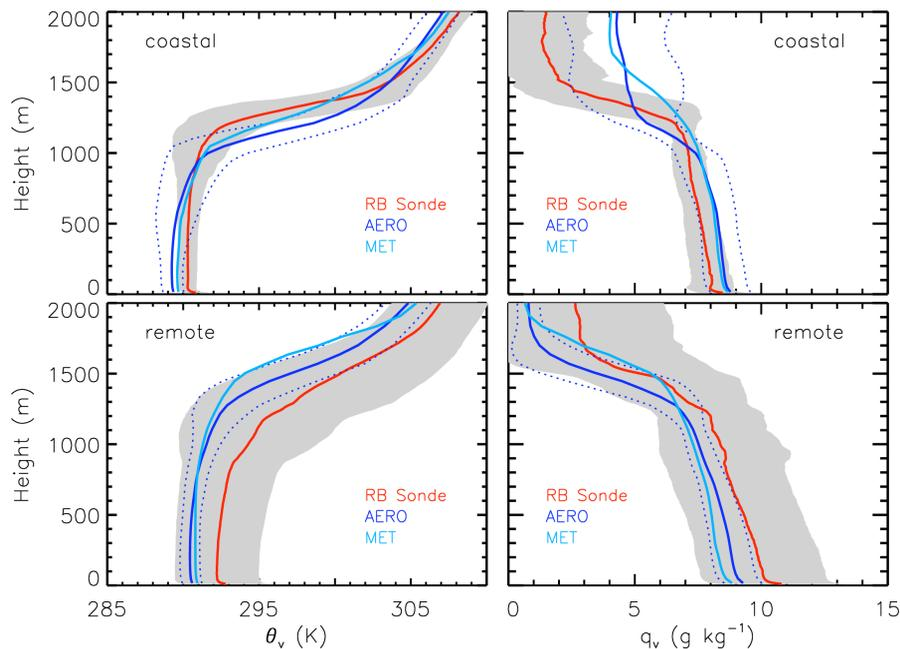
**Fig. 1.** Vertical profiles of virtual potential temperature ( $\theta_v$ ) and water vapor mixing ratio ( $q_v$ ) measured by radiosondes released from the RB ship and those from AERO (blue) and MET (light blue) simulations. The shaded area represents  $\pm 1\sigma$  of the observations. The dash blue lines also indicate the  $\pm 1\sigma$  of the AERO simulations.
