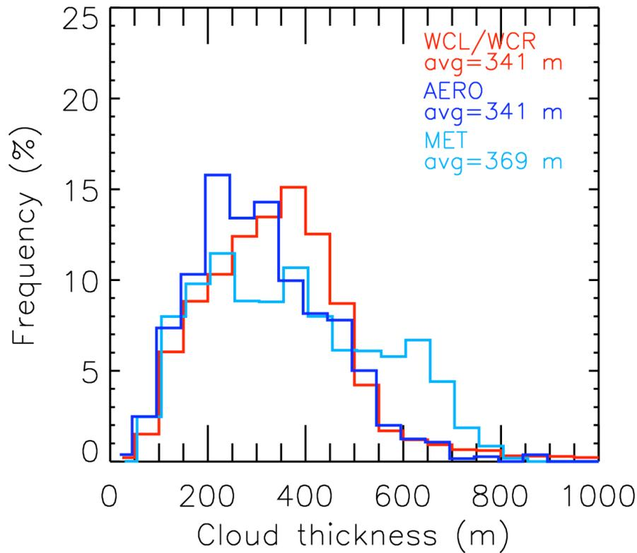
**Fig. 8.** Histogram of cloud thickness from the Wyoming cloud lidar (WCL) and radar (WCR) observations (red), and from the AERO (blue) and MET (light blue) simulations.
