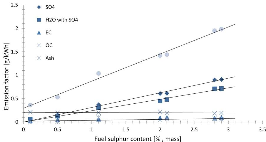
**Fig. 3.** The emission factor of the total PM, and for its chemical constituents as a function of fuel sulphur content (mass-based percentage), based on the data from the second IMO GHG study (Buhaug et al., 2009). Linear regression curves are presented as black lines. The emission factors of the total PM,  $\text{SO}_4$  and  $\text{H}_2\text{O}$  are linearly dependent on the fuel sulphur content. The data points for EC and ash are partly overlapping in the figure.
