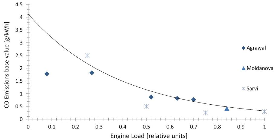
**Fig. 5.** The base value of CO-emission as a function of relative engine load. The measurements of Agrawal, Moldanova and Sarvi have been shown, and the CO-base emission factor curve is based on Sarvi. The emissions of CO are also influenced by rapid changes of relative engine load.
