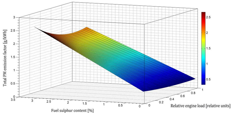
**Fig. 4.** The predictions of the STEAM2 model for total PM emission factor [legend, in units of  $\text{g kWh}^{-1}$ ] as a function of engine load and fuel sulphur content.
