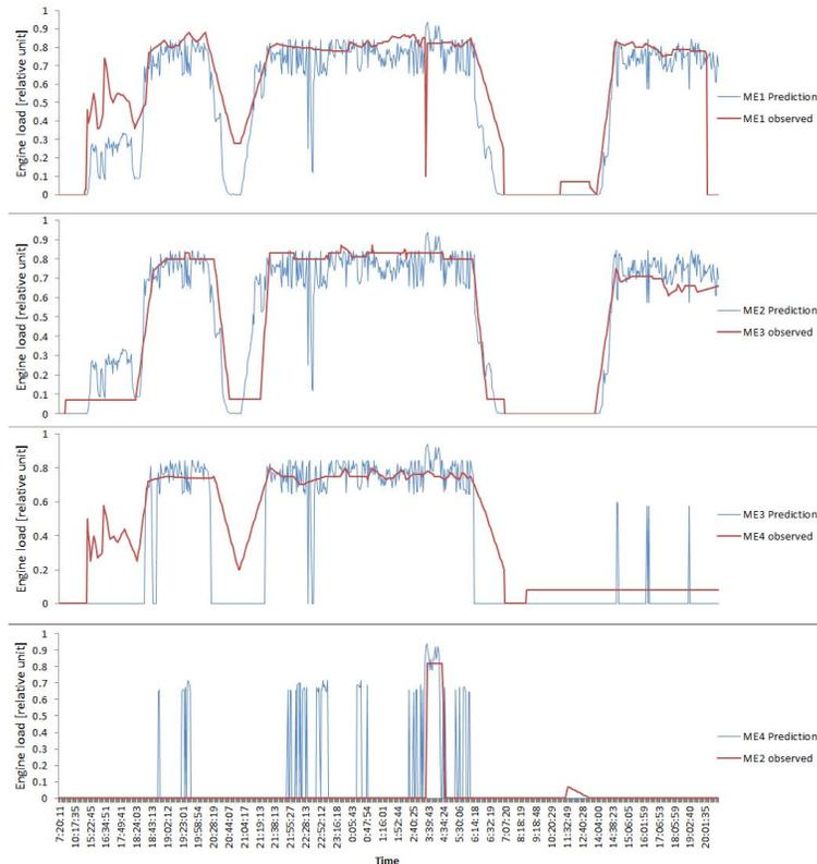
**Fig. 9.** Predicted and observed engine loads of four identical main engines in a large RoPax ship. The time scale for all plots (a–d) is the same, presented in (d). MEx,  $x = 1, 2, 3, 4$ , are the four main engines. The numbering of the main engines in the model has no influence on the engine load predictions; for instance, in (b) the curves ME2 (estimate) and ME3 (observed) are directly comparable.
