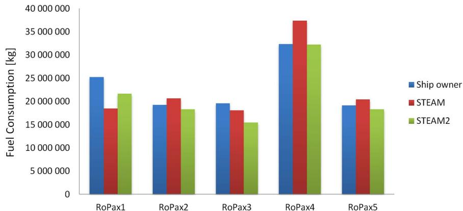
**Fig. 8.** The reported and predicted total fuel consumption for five RoPax vessels from January to November in 2007. The vessel RoPax 4 is the same ship, the data of which has been presented in Fig. 7a–b.
