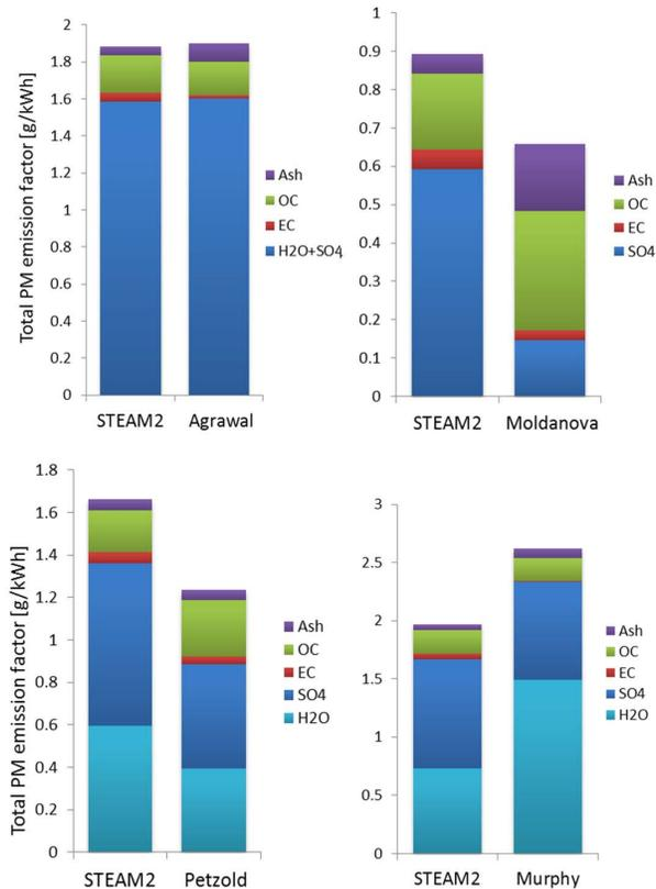
**Fig. 10.** Comparison of the predicted and measured emission factors for the chemical constituents of PM. The measured data has been extracted from Agrawal et al. (2008b), Moldanova et al. (2009), Petzold et al. (2008) and Murphy et al. (2009).
