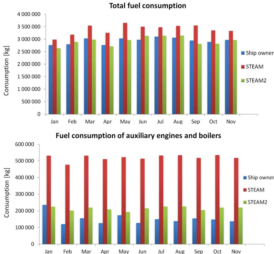
**Fig. 7.** The monthly average fuel consumption of a RoPax ship in 2007, as reported by the ship owner, and predicted by the two model versions. The total fuel consumption is presented in the upper panel, and the fuel consumption of auxiliary engines and boilers in the lower panel.
