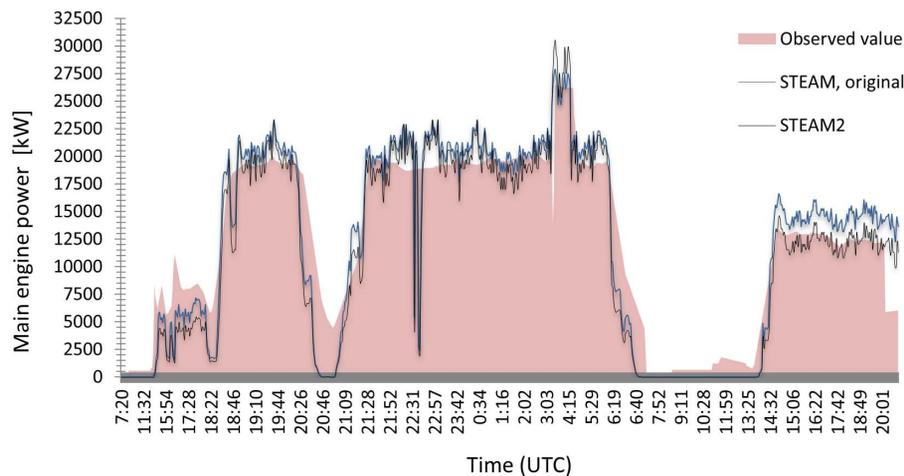
**Fig. 6.** The predictions of the STEAM and STEAM2 models and the corresponding measured engine power. The data has been measured for a 60 000t RoPax vessel that was sailing in the Baltic Sea within and near the archipelago surrounding the city of Stockholm in April 2008.
