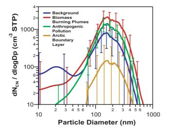
**Fig. 2.** Average dry particle size distributions for each air mass type sampled during 12–21 April. Error bars denote one standard deviation from the mean.
