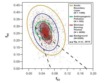
**Fig. 8.** Oxidation state of the aerosol expressed as  $f_{44}$  versus  $f_{43}$ , following Ng et al. (2010). Points denote the 5-min-averaged observations for each air mass type, and the ellipses denote the 95 % confidence regions. Dashed lines are the parameterized triangular bounding region reported by Ng et al. (2010) for SOA chamber oxidation and ambient measurements.
