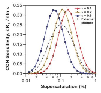
**Fig. 9.** Sensitivity of  $R_a$  to  $\kappa$  as a function of superaturation. Solid traces were computed assuming an internal mixture and constant values of  $\kappa$ , while the dashed trace represents an external mixture of 50% inorganic aerosol ( $\kappa$  = 0.6) and 50% organic aerosol ( $\kappa$  = 0.1), by number.
