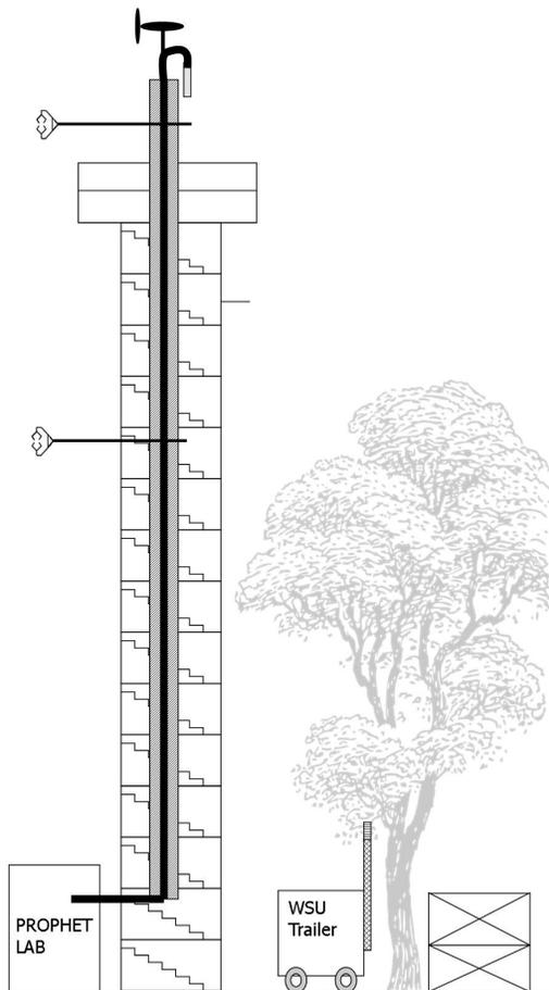
**Fig. 1.** University of Michigan Biological Station (UMBS) PROPHET tower schematic as configured for CABINEX 2009. Two sonic anemometers were used for this study: “top” at 34 m (1.5 canopy height) and “mid” at 20.6 m (0.92 canopy height).
