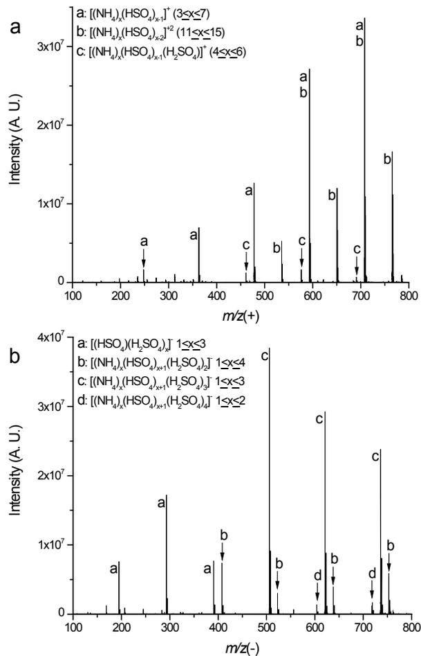
**Fig. 1.** Electrospray ionization mass spectra of an ammonium sulfate solution in **(a)** positive and **(b)** negative modes.
