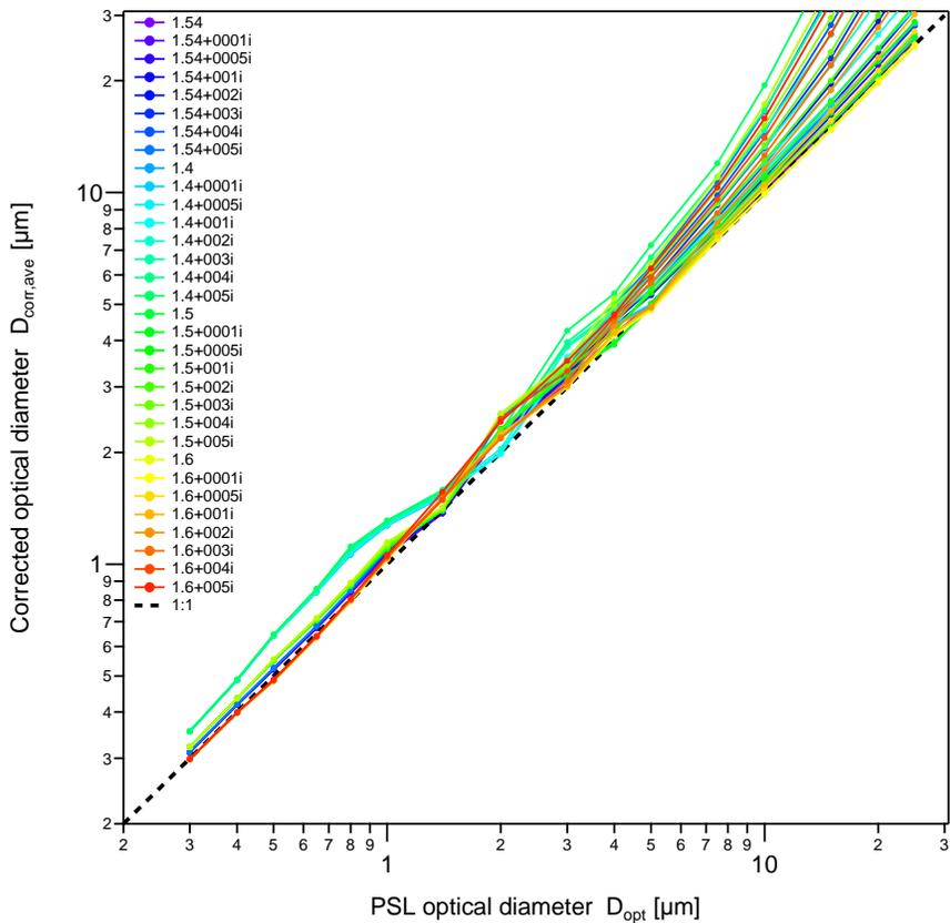
**Fig. 19.** Diameter correction curves for the deployed Grimm 1.108 OPC for a selected matrix of complex refractive indices.
