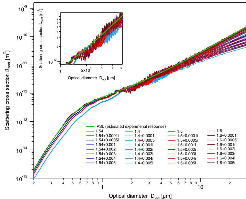
**Fig. 17.** Calculated scattering cross section versus the optical diameter for different refractive indices (see legend), considering the technical details of the used OPC (see text for details).
