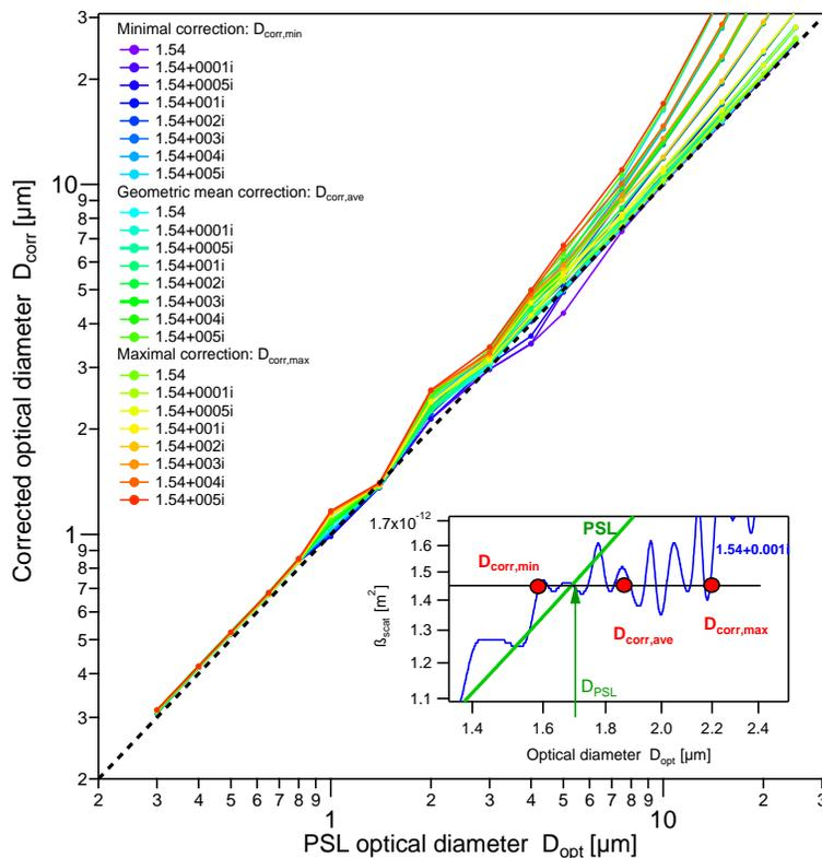
**Fig. 18.** The Figure shows OPC diameter correction curves for a complex refractive index of  $1.54 + 0.005i$ . Due to the wiggled shape of the curves shown in Fig. 17, the diameter correction is not bijective. Therefore, minimal, geometric mean as well as maximal correction functions are shown (see illustration in the Figure inset).
