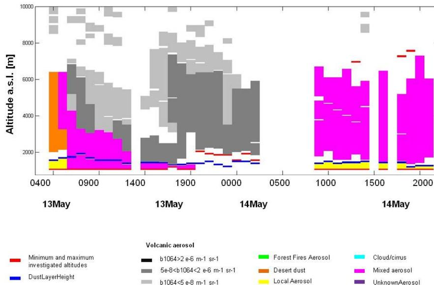
**Fig. 6.** Aerosol mask for the 13–14 May 2010 case as obtained by the methodology reported in this section. Only the time window affected by volcanic aerosol is included.
