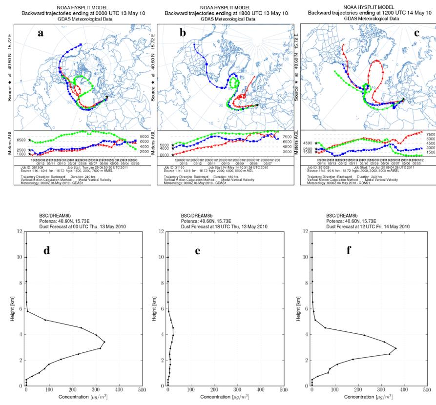
**Fig. 3.** HYSPLIT backtrajectory analysis (upper panel) and DREAM forecast vertical profiles of dust concentration (lower panel) for 13 May, 00:00 UTC (**a, d**), 13 May, 18:00 UTC (**b, e**) and 14 May, 12:00 UTC (**c, f**). Altitude layers at arrival point in the backtrajectory analysis are chosen accordingly to the layers identified through the method reported in Sect. 3.1.
