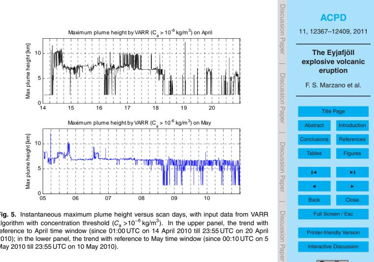
Fig. 5. Instantaneous maximum plume height versus scan days, with input data from VARR algorithm with concentration threshold ( $C_a > 10^{-6} \text{ kg/m}^3$ ). In the upper panel, the trend with reference to April time window (since 01:00 UTC on 14 April 2010 till 23:55 UTC on 20 April 2010); in the lower panel, the trend with reference to May time window (since 00:10 UTC on 5 May 2010 till 23:55 UTC on 10 May 2010).
