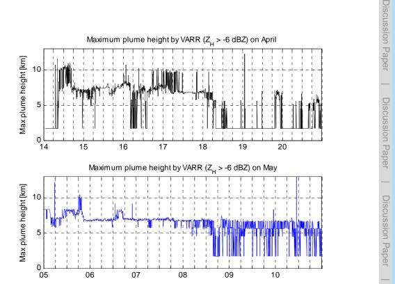
**Fig. 6.** Instantaneous maximum plume height versus scan days, with input data from VARR algorithm with reflectivity threshold ( $Z_{\rm H} > -6$  dBZ). In the upper panel, the trend with reference to April time window (since 01:00 UTC on 14 April 2010 till 23:55 UTC on 20 April 2010); in the lower panel, the trend with reference to May time window (since 00:10 UTC on 5 May 2010 till 23:55 UTC on 10 May 2010).
