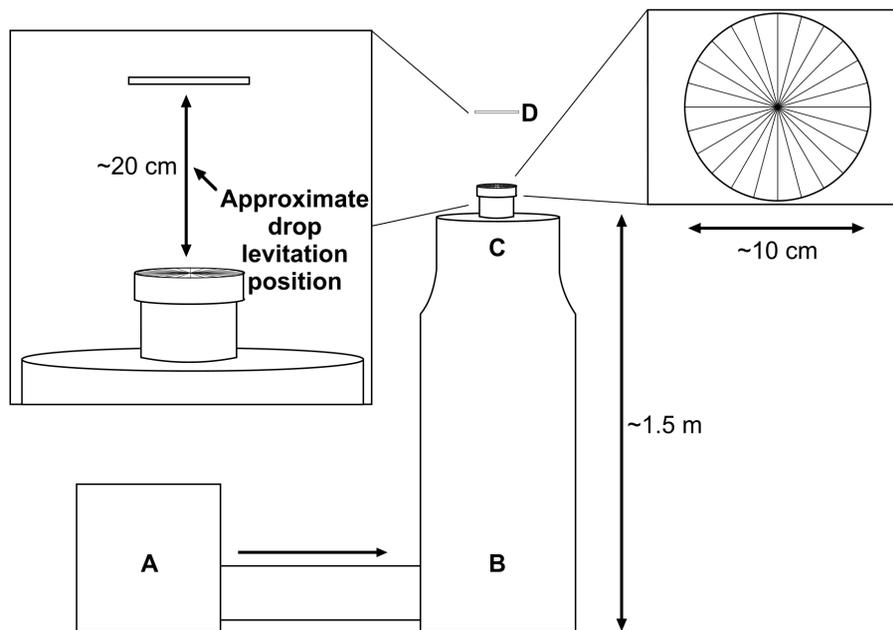
**Fig. 1.** Experimental setup; vertical wind tunnel: fan (A) blows air through into settling chamber (B) to minimise turbulence before exiting through top orifice (C). Orifice is covered with a wire grate to produce a radial pressure profile which in conjunction with top plate (D) provides a back-pressure and creates a stagnation well in which drops can levitate.
