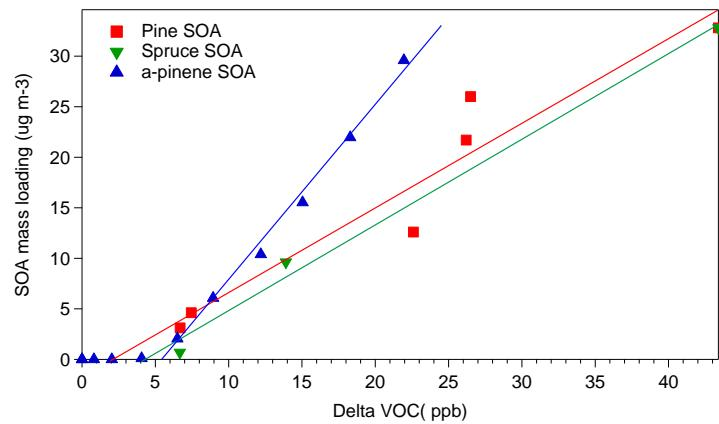
Fig. S2 Aerosol mass concentration as a function of the terpene concentration for emissions of pine (red), spruce (green) and a-pinene (blue).
