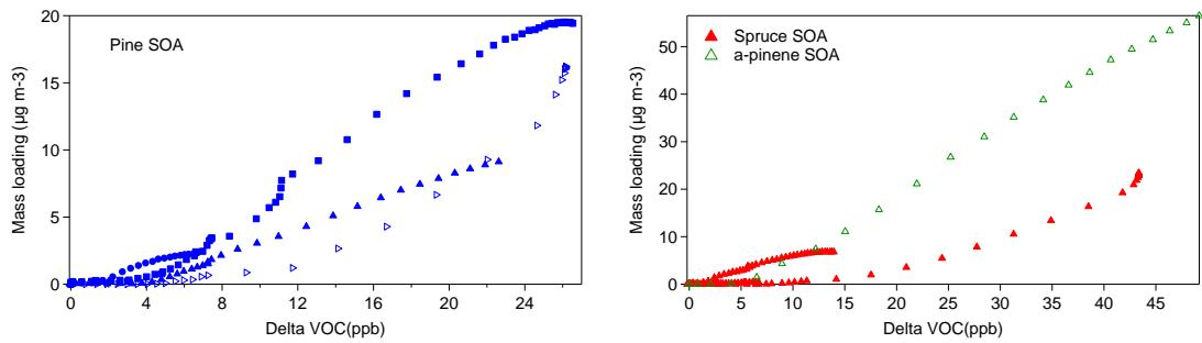
Fig.S1 Growth curves for a-pinene and real plant SOAs in this work.
