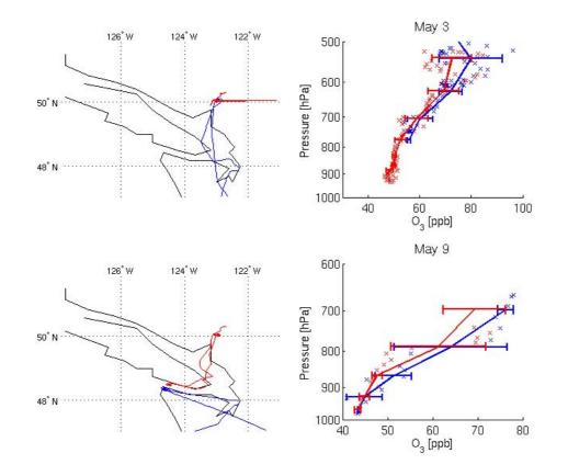
**Fig. 2.** Flight tracks and vertical mean profiles of ozone measurements during the two intercomparison flights between the C-130 (shown in blue) and the Cessna (in red). Top panels show the May 3 flights; bottom panels show the 9 May flights. Crosses indicate 1-min mean measured values of ozone on each platform. Data are filtered to include only points where the two platforms flew within 0.3° latitude and longitude of one another.
